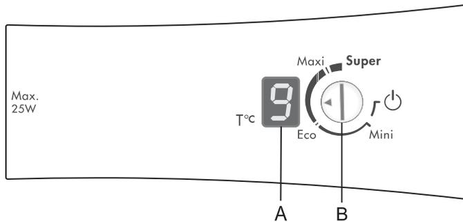
**A Digital temperature display** (certain models only) of the refrigerator indicates actual temperatures during the operation from +1°C to +9°C
