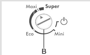
The appliance is switched on by turning the button (B) towards **Maxi**, and accordingly switched off when the arrow (small triangle) on the button points to the ON/OFF mark  $\Phi$  (the appliance, however, is still under mains power).
